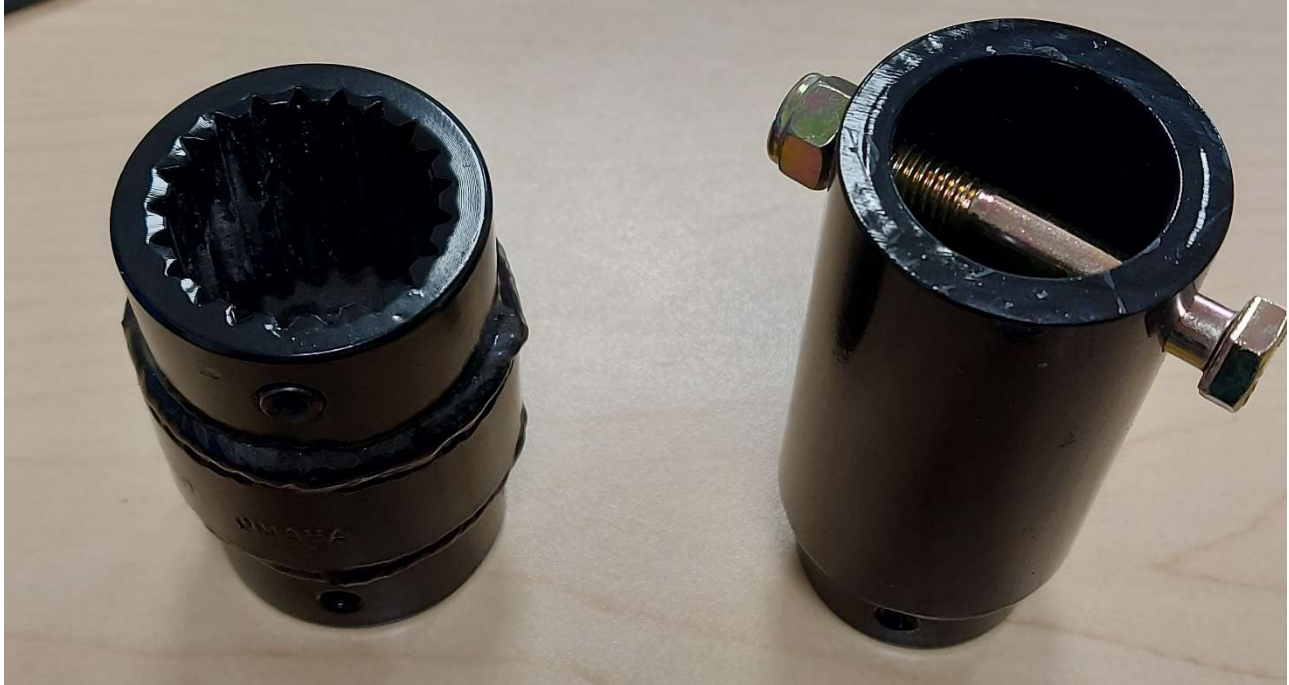
Figure 3 Motor Couplings (21 Spline & Cross Bolt)
