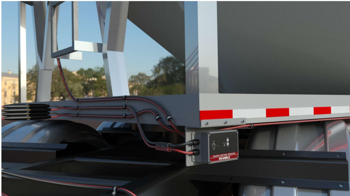
Figure 4 Telescopic Tarp Arm Control Box Mounting
