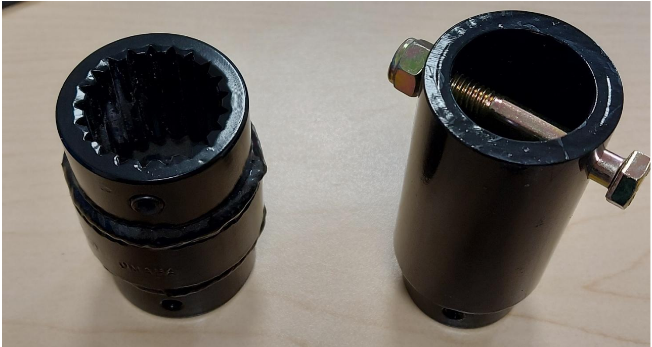
Figure 3 Motor Couplings (21 Spline & Cross Bolt)
